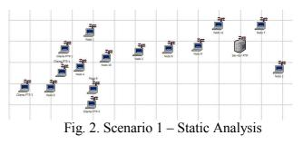
There are four client nodes which download a 100 KB file from a FTP server 20, 30, 40 and 50 seconds after the simulation starts, respectively. Just 400 seconds after that download, each client starts again with the same download process, which is repeated every 50 seconds.
